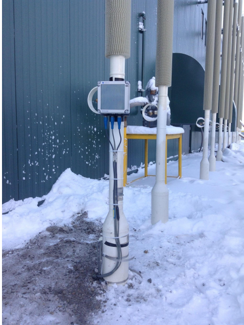
Armored Data Temperature Cables connected to a D405 Logger mounted on a thermosyphon
