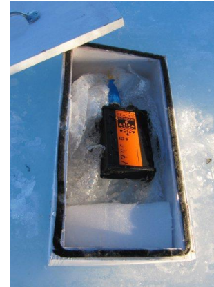
A close-up of a beadedstream digital temperature cable connected to a DL230 Data Logger. This logger provides reliable temperature data collection with extreme low power consumption and safe onboard flash storage at Wilkins Aerodrome.
