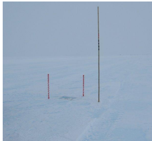
One of the digital temperature cables installed in the runway ice.
