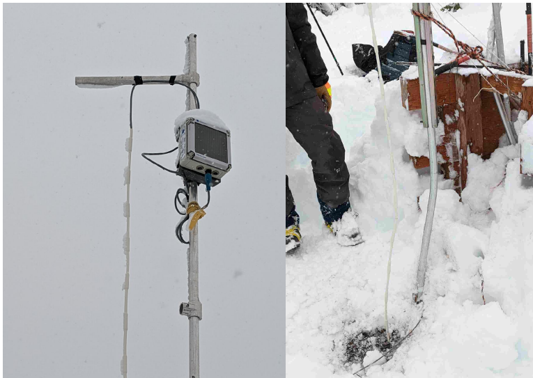
Left - D405 logger with temperature cable in white heat shrink.
