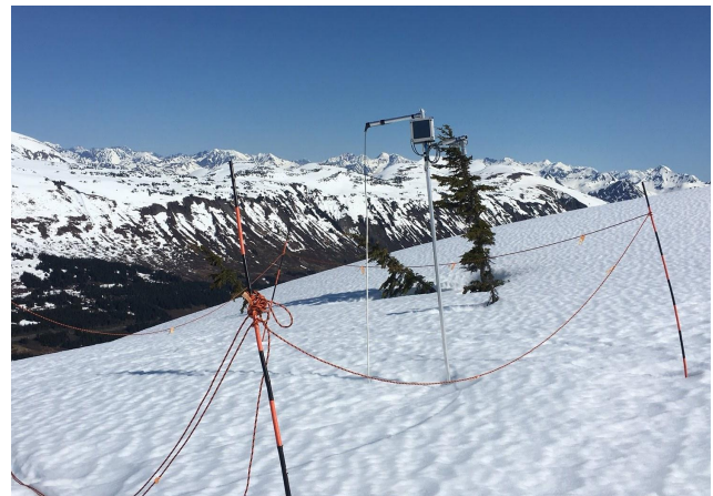
D405 Data Logger mounted on top of a post during low snow conditions. The temperature cable can be seen suspended from the arm to the left of the post.
