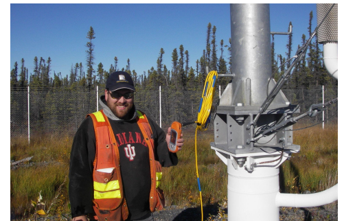
A field data collector at the HAARP Station showing beadedstream's Digital Temperature Cable and a hand-held readout device.
