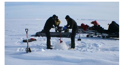
Installation of beadedstream Digital Temperature Cable at Teshekpuk Lake.
