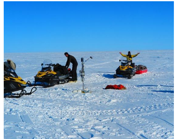
An ALISS buoy retrofitted with beadedstream D405 data logger deployed into a lake during the summer.
