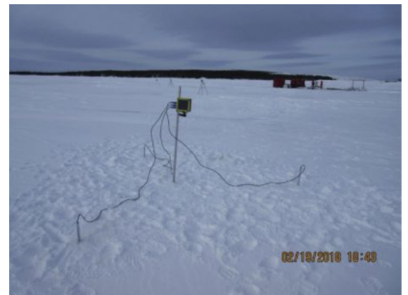
Three temperature probes connected to a D405 Logger on frozen sea ice.
