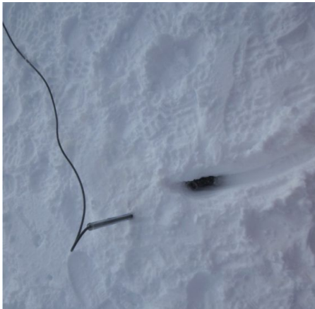
Snow pit adjacent probe being used to measure snow thickness on the sea ice
