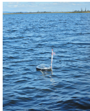
A buoy deployed into a lake prior to freezing (left) and after (right). The 0.4m (1.3 ft) of air sensors are visible above the surface.
