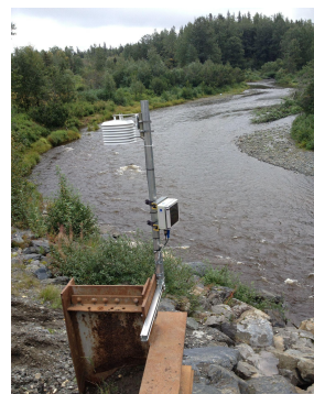
Monitoring Stations located at Anchor River (left) and Deshka River (right) showing the D405 Data Logger and air temperature sensor mounted to a post.
