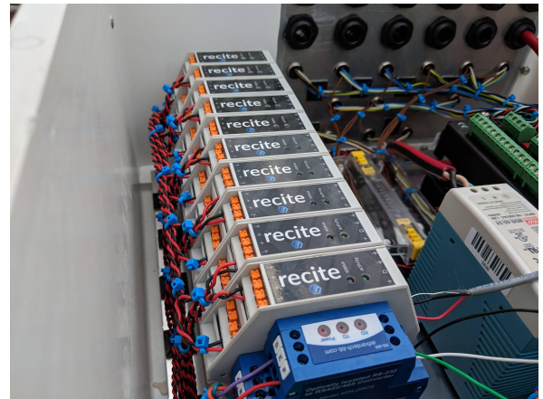
Recite interfaces inside a Campbell Scientific Data Logger enclosure.
