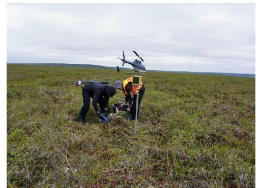
beadedstream team installing temperature monitoring gear at a snow station in the tundra
