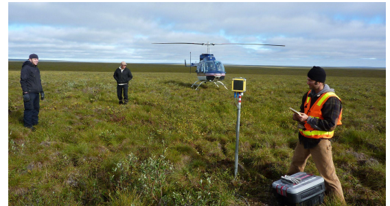
beadedstream team installing digital thermistor strings and a data logger at a tundra monitoring station, with a helicopter in the background.
